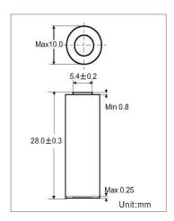
Chemical System: Primary Alkaline Camelion No.: 23A Average Weight: 7.9g Dimension (Ø xH): 10.0 x28.3 mm Terminals: Flat Nominal Voltage: 12.0Volts Nominal Service Capacity: 55mAh (20±2°C, Rated at 20kΩ load to 6.0V) Jacket: Metal Label Operating Temperature: -20°C~54°C Cross Reference: EL12(Japan), VR22(Ranson)
