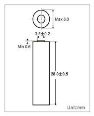
Chemical System : Primary Alkaline Camelion No.: 27A Average Weight : 4.6g Dimension ( $\emptyset$  xH) : 8.0 x28.5 mm Terminals : Flat Nominal Voltage : 12.0Volts Nominal Service Capacity: 16mAh ( $20\pm2^{\circ}$ C, Rated at 20K  $\Omega$  to 7.2V) Jacket : Aluminum Foil Label Cross Reference: EL-812(Japan), B-1(Bronica)
